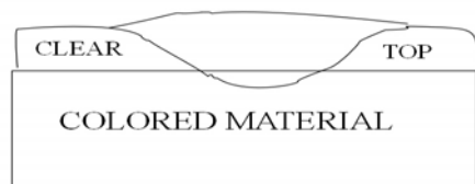
2nd FILL - SLIGHT OVERFILL
