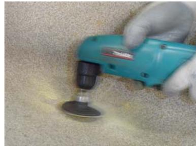
**Remove blister area by cutting and grinding**
